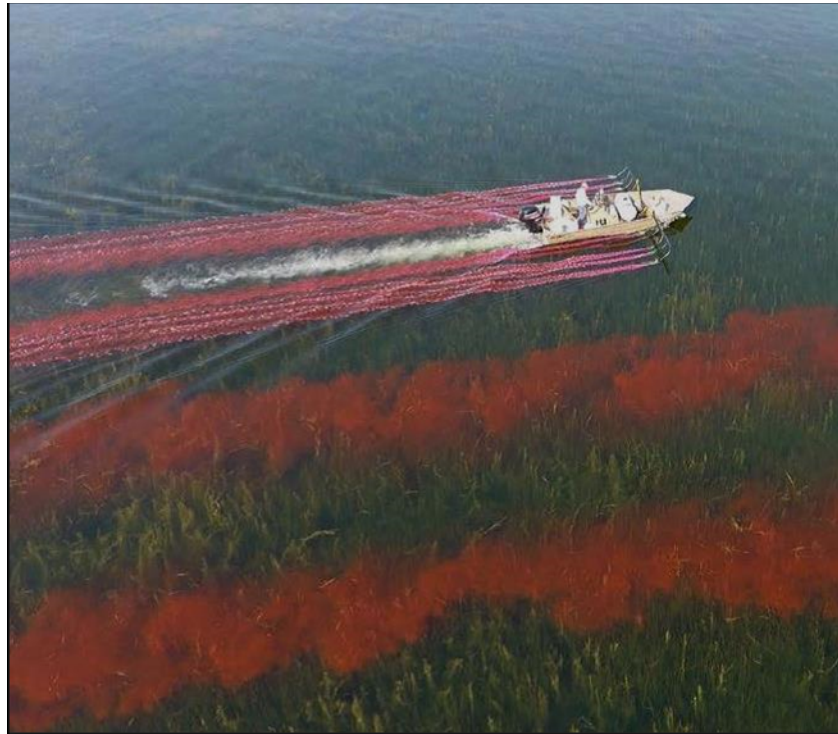
Figure 1. Subsurface application of rhodamine water tracer (RWT) to an open-water stand of submersed plants to simulate an aquatic herbicide application, Lake Pend Oreille, Idaho.
